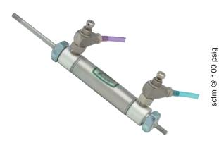
Clippard offers five models of adjustable flow controls with #10-32 through 3/8" NPT ports. They feature a combination needle and check valve that controls flow in one direction and allows free flow in the opposite direction.
